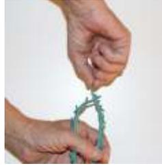
Flex the belt further and insert the 2nd tab through the end link by twisting it with your thumb.
