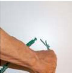
Hold the belt ends together with the tabs pointing outward.
