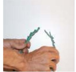
Pull the belt end with the tab through two links to separate the belt pieces.
