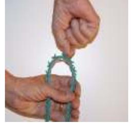
Insure the tab returns to position across the belt. Reverse the belt so the tabs run inside.
