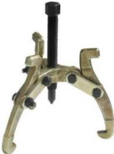
The tool to the left is called a “gear puller”, the easiest way to remove a stuck pulley without damaging the arbor and motor. They are fairly inexpensive, and if you can’t borrow one, are a bargain compared to buying a motor.
